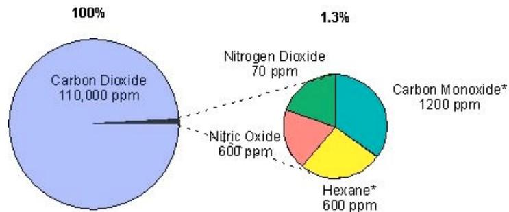
\*Automobile Catalytic Converters Convert These Gases To Carbon Dioxide
