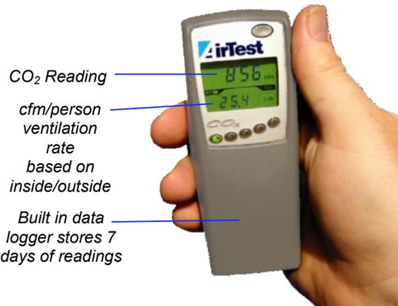
The PT9250 CO<sub>2</sub> & Ventilation Rate Monitor
